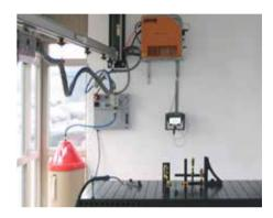
The **KEMPER VacuFil Compact** is equipped with an extra large, vertically mounted filter cartridge for particularly effective cleaning. The separation efficiency is more than 99.9 % and effectively protects welders in industrial applications against the finest particles in welding fumes.
