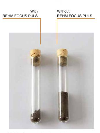
Welding fume emission when welding 1 kg of solid wire.
